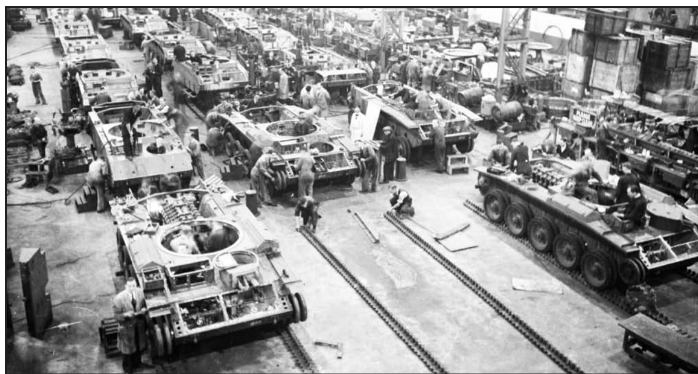
● Crusader Tank's being made in their secret locations in Britain PHOTOGRAPH SUPPLIED BY THE IMPERIAL WAR MUSEUM
